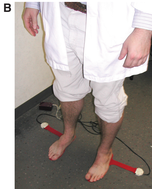
Figure 3. A, Pedar sensors are connected via wireless interface and are used to measure plantar pressures. B, Shifts in pressure are converted into shifts in center of pressure to evaluate the stability of the test patient after a “push.”
